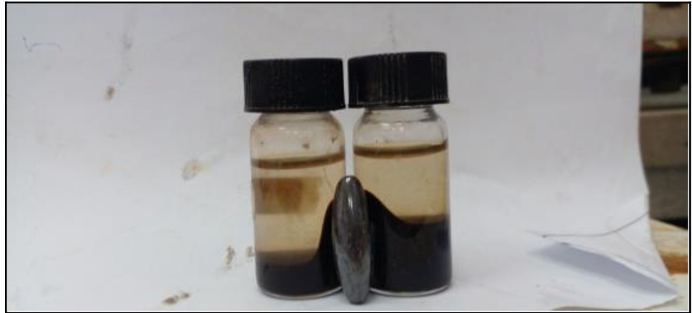
Fig 2. Extracted Fe-NPs from peels of banana, pomegranate, opuntia, orange, potato, and onion under an external magnetic field.
