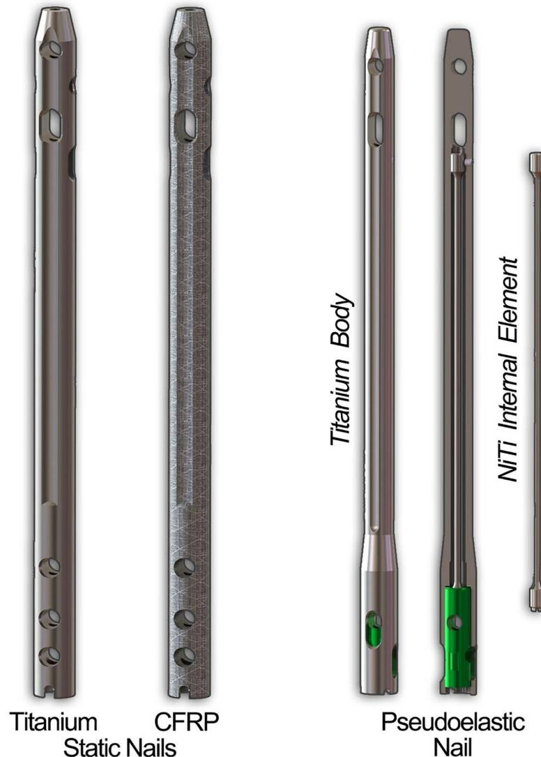
**Fig 1. Renderings of the three IM nails used in this study.** The static nails were modeled after a 10 mm VersaNail using both titanium and CFRP material properties, while the DynaNail represented a dynamic nail with an internal NiTi element inside a titanium outer body.
