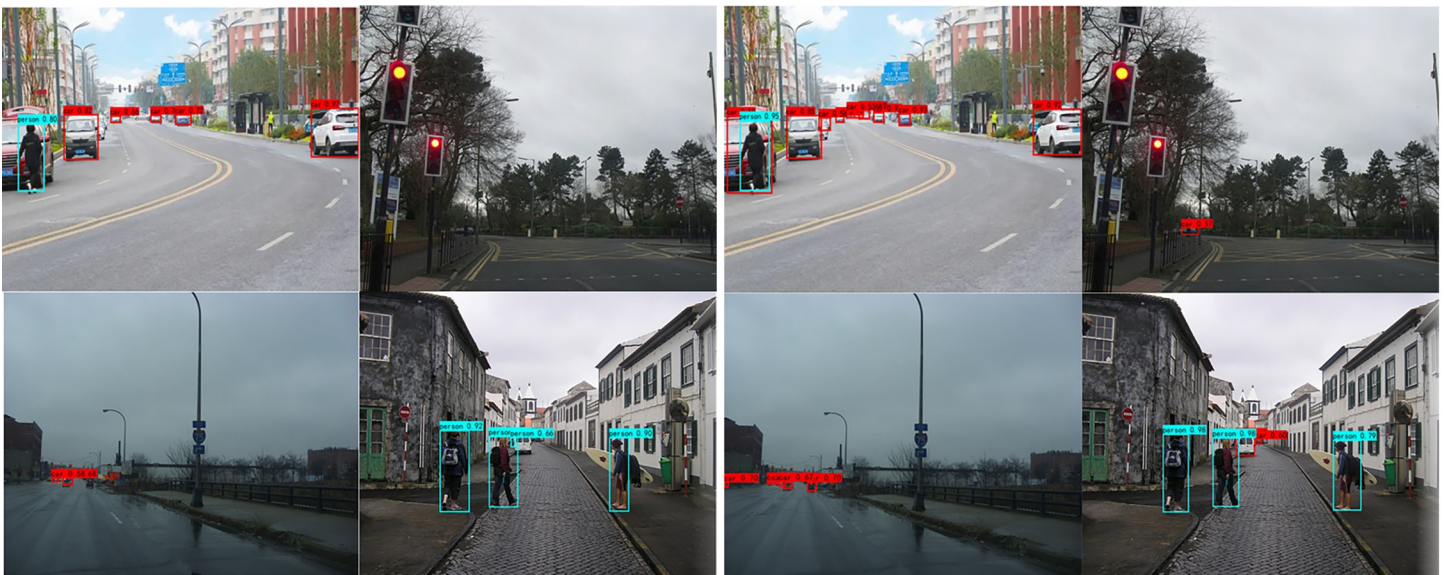
Fig 12. Comparison of the detection effect of SwinT-YOLOv4 and YOLOv4. (A) Detection effect of YOLOv4; (B) Detection effect of SwinT-YOLOv4.
