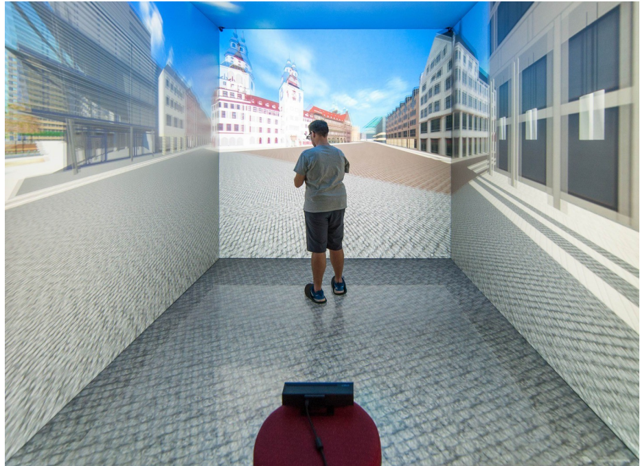
Fig 2. The virtual reality study setup showing the experimental setup in the virtual city center of Chemnitz, Germany inside the five-sided cave automatic virtual environment.
