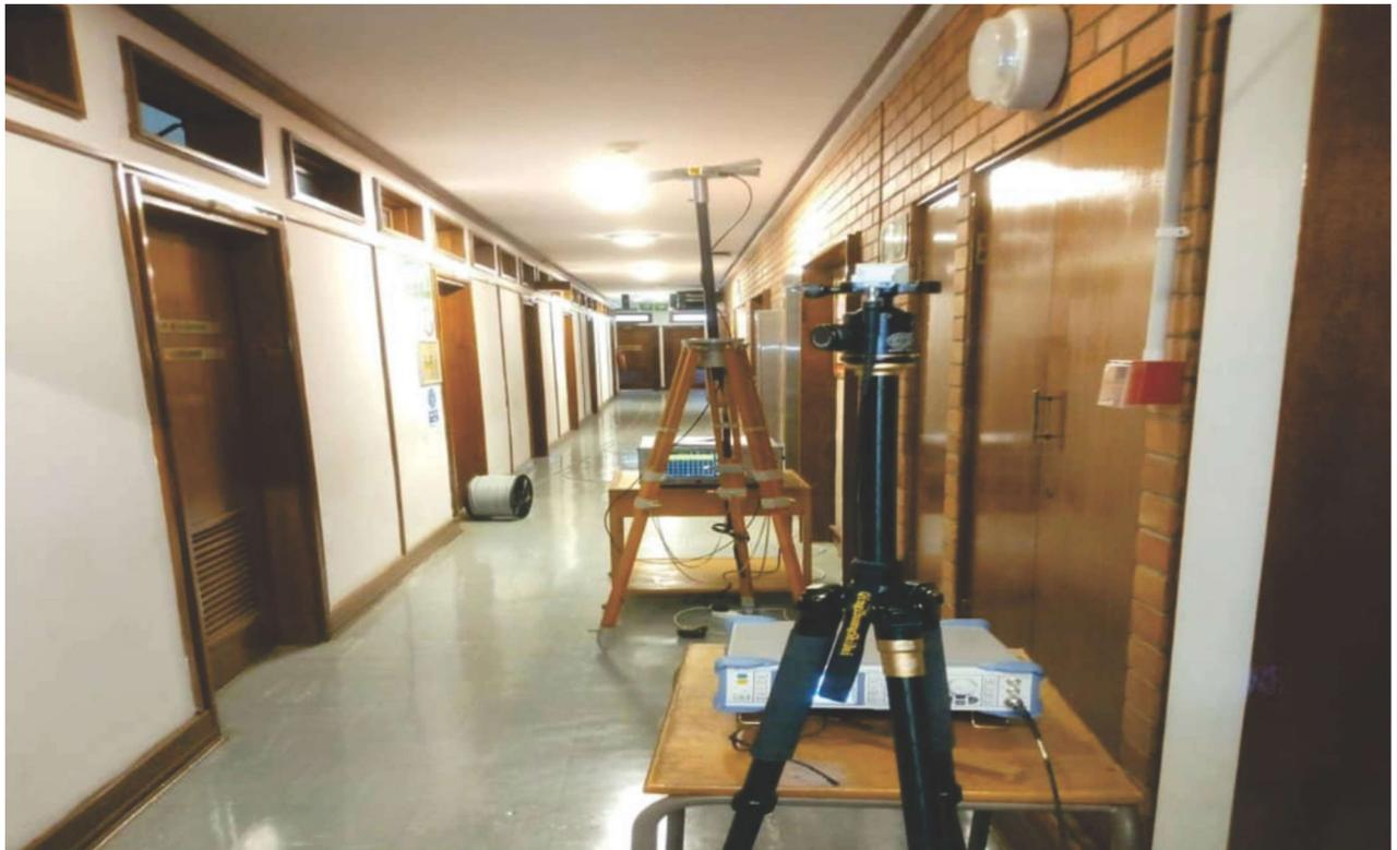
**Fig 6. The setup of the Tx and the Rx in the indoor corridor environment.**
