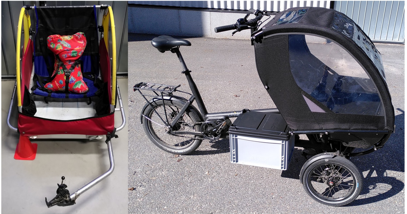
Fig 1. Test vehicles for child transport used in this study: Cycle carrier Kinderkar with dummy (left) and Cargotrike Chike.
