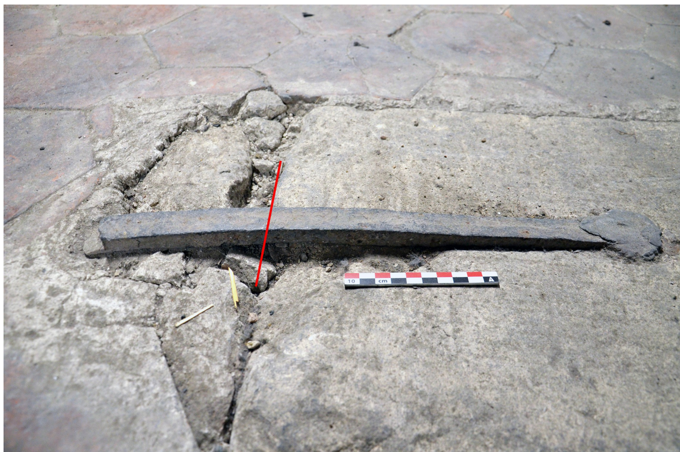
Fig 6. Broken staple in the tribunes (TRIB01S). The red line indicates the sampling. The sample was then cut longitudinally for analysis.
