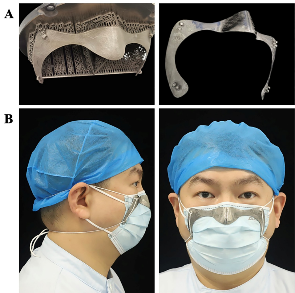
Fig 3. Surgical mask retainer. Panel A shows fabrication of the retainer by using 3D printing technology before and after support was removed. Panel B shows participant wearing surgical mask supplemented by the retainer.
