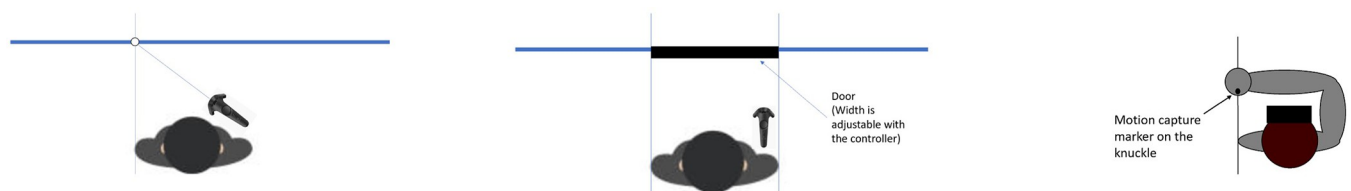
Fig 7. Test 1—Visually measuring the position of the real shoulder. A. A wall of height 3m appeared 1m in front of each participant parallel to their bodies (shoulders) and the avatar was made invisible. On the wall, a horizontal straight line appeared at a random height within the range of \pm 10 cm vertically from the shoulder position of the participant (shoulder height was read from the motion capture marker pasted on the shoulder of the participant). A controller was handed to the controlled hand of each participant, and they were asked to point on the line, the position that corresponds to the edge of their non-controlled shoulder. Here the figure shows the ideal case in which the right participant points perfectly at the edge of their left shoulder. The task was opposite for the left participant, who had to use his left hand to point to his right shoulder. B. Test 2—Measuring the width of the real body. A wall of height 3m appeared 2m in front of the participants and the avatar was made invisible. On the wall a door of height 2m and width 30 cm appeared within the range of \pm 10 cm horizontally from the center of the body. Using the touch pad buttons of the controllers given to each participant, they were asked to adjust the width of the door to match the width of their real bodies. This figure demonstrates a perfectly matched scenario. C. Test 3—Measuring the proprioceptive position of the shoulder. During this test, the HMD was blacked out to avoid the participants seeing anything in VR or their real bodies. They were asked to move their controlled arm hand to place the motion capture marker on the knuckle of that hand just in front of the end of the shoulder of the non-controlled arm shoulder of their real bodies (participants were asked to remember the position of the specific motion capture marker pasted on the knuckle of the controlled arm before the experiment started). They were instructed to make the localization in one smooth movement and not to touch/search for the shoulder. This figure demonstrates a perfectly pointed scenario.
