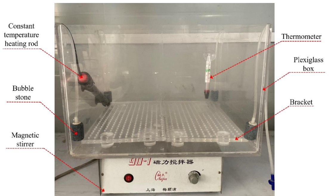
Fig 3. Device for immersion curing.
