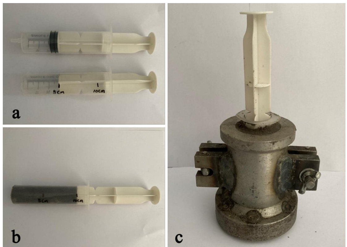
Fig 5. Shaping of specimens with mixed bacteria.
