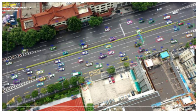
Fig 3. Video processing by using the automated roadway conflicts identification system.
