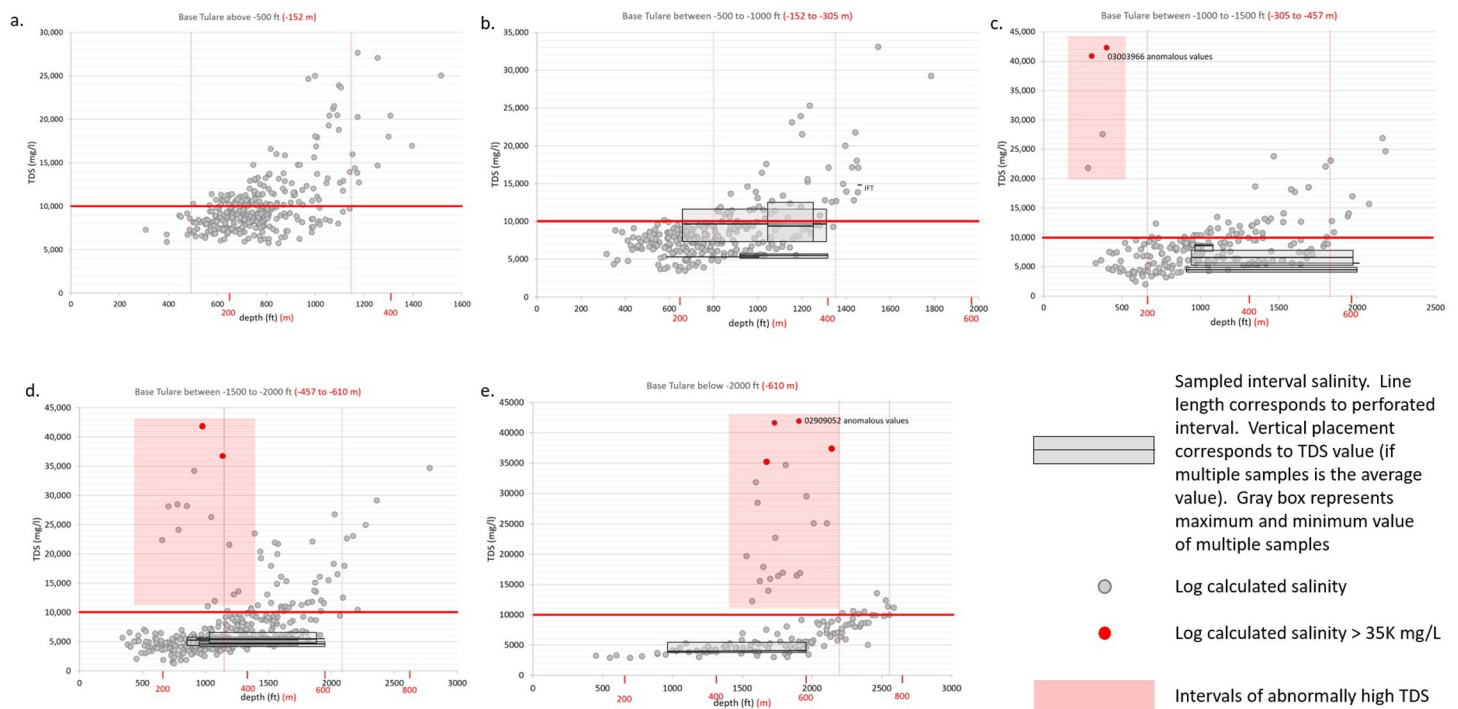
Fig 8. Log-calculated total dissolved solids (TDS) versus depth plots for wells within different elevation ranges for the base of the Tulare Formation. Log calculated TDS shown by the gray dots. Wells with lab sample analyses are shown as black horizontal lines between the upper and lower perforated interval depths. The vertical position of the line corresponds to the salinity value of the sample. For wells with multiple samples, the highest and lowest salinity values are shown by a gray box and the horizontal line is placed at the average salinity value. Red boxes note log calculated salinity values that are abnormally high and are sometimes associated with produced water disposal wells. The red horizontal line on each graph marks the 10,000 mg/L TDS value. Red vertical dashed lines mark the upper and lower depths at which groundwater salinity exceeds 10,000 mg/L within each depth range. Points with calculated salinities greater than sea water are shown in red. Values in feet in black, values in meters in red.
