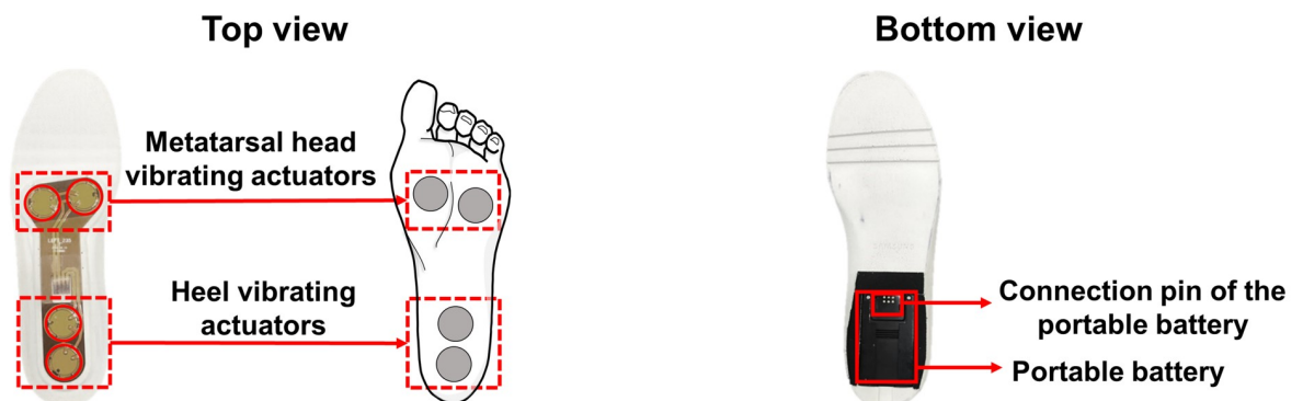
Fig 1. Overview of the components of the shoes and vibrating insole that apply mechanical vibration. (A) The components of the shoes that apply the mechanical vibration to the soles of the feet. The main components are the vibrating insoles that contains the actuators that deliver mechanical vibration, a foam sole placed on top of the insoles to act as a shock absorber, and main body of the shoe that contains the connection pin and charging port to recharge battery. (B) The top and bottom view of the vibrating insoles. The top view shows the position of pair of actuators used to deliver the vibration to the metatarsal head (front actuators) and heel (rear actuators). The amplitude of the vibration is controlled independently for the two pairs of actuators, which allows users to apply the vibration to different areas of the foot with different amplitudes. The bottom view shows the position of the portable battery and the connection pin for the charging port of the shoes.
