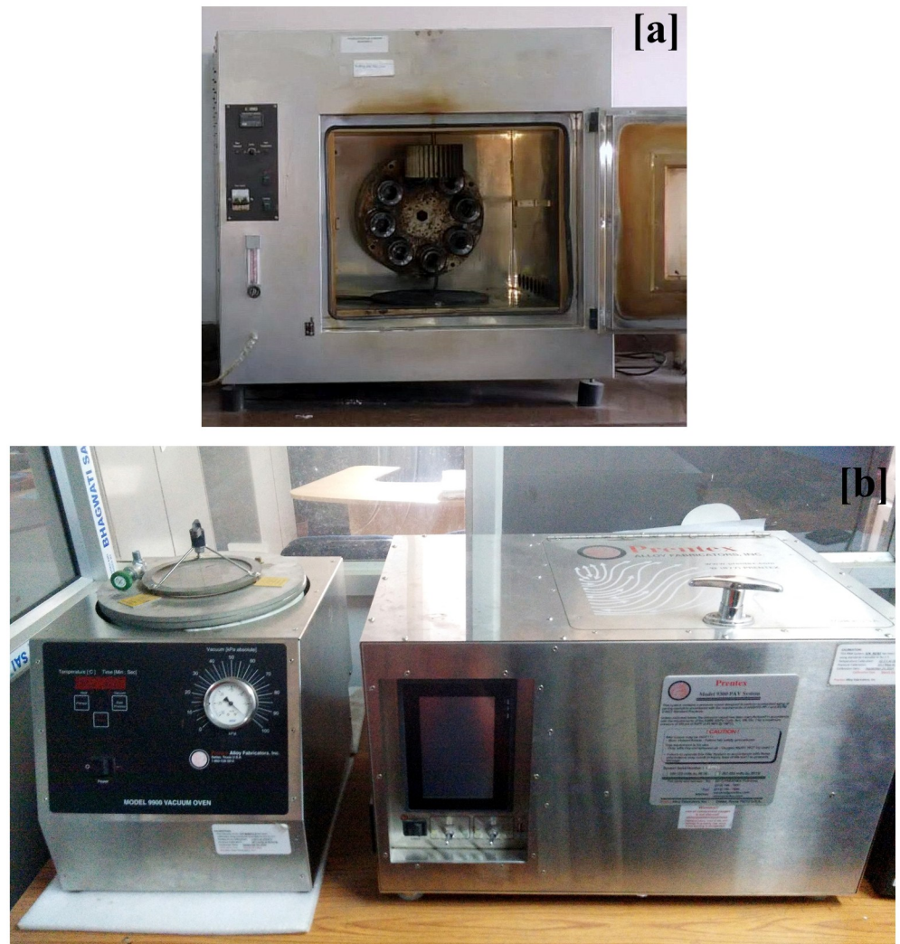
Fig 3. (a) RTFO device used for simulation of short-term aging, and (b) PAV device used for simulation of long-term aging.
