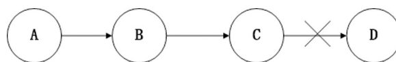
Fig 1. Routing maintenance example: Node C cannot forward the packet of node A to the next hop of the route.
