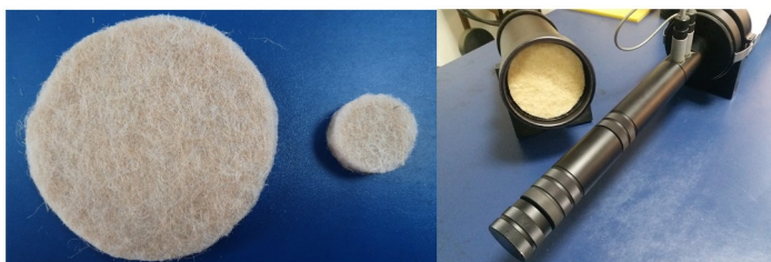
Fig 4. Jute fiber felt samples and the impedance tube installed with a sample.
