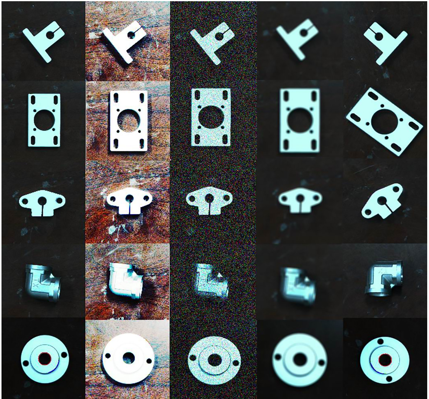
Fig 6. Part of the object in the dataset (from left to right: The original image of the object, image after shading adjustment, the image with Gaussian noise, blurred image, and rotation image).
