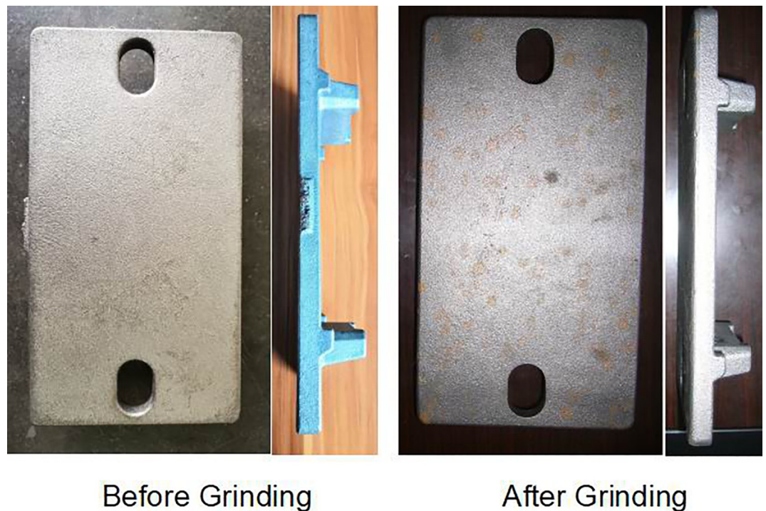
Fig 18. Picture showing the object before (left) and after (right) grinding (the burr on the workpiece surface is cleanly removed).
