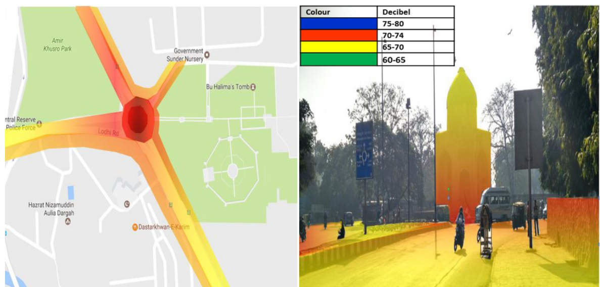
Fig 8. 2D & 3D Noise mapping of Sabz Burj. The colors indicates the different noise zones. Blue: maximum noise level 75-80dB (A); Red: maximum noise level 70-74dB (A); Yellow: maximum noise level 65-70dB (A); Green: maximum noise level 60-65dB (A). A version of this figure with the original imagery is available from the authors.
