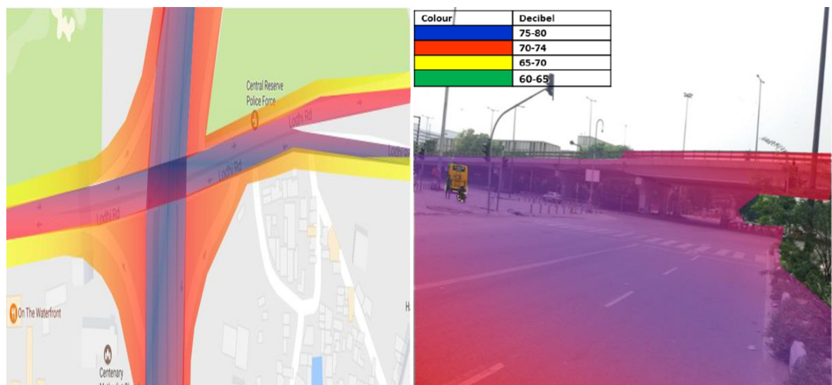
Fig 9. 2D & 3D Noise mapping of Loadhi road. The colors indicates the different noise zones. Blue: maximum noise level 75-80dB (A); Red: maximum noise level 70-74dB (A); Yellow: maximum noise level 65-70dB (A); Green: maximum noise level 60-65dB (A). A version of this figure with the original imagery is available from the authors.
