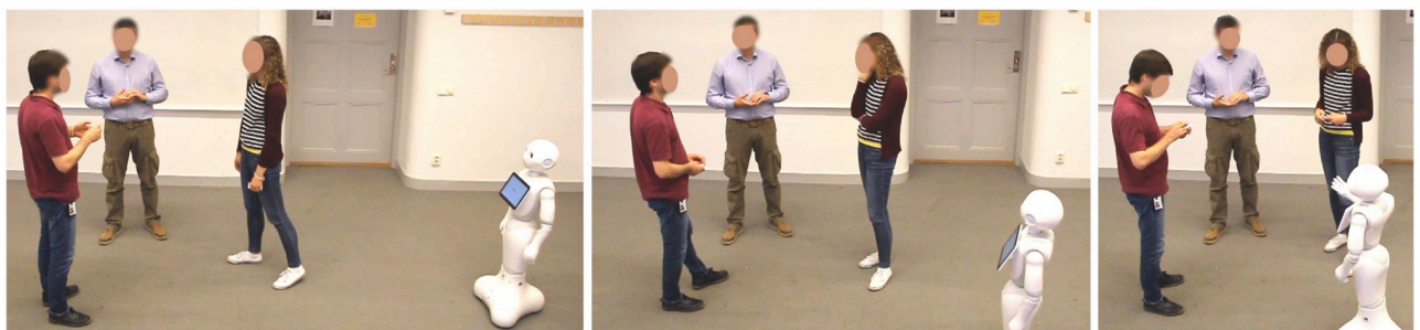
Fig 1. A representative image of the encounters captured in the CongreG8 dataset. In this case, a Pepper robot approaches a free-standing conversational group in order to join it. The complete dataset consists of trials of human approach behaviors and robot approach behaviors. Actual recordings took place in a motion capture facility in which all participants (apart from Pepper) wore motion capture suits.
