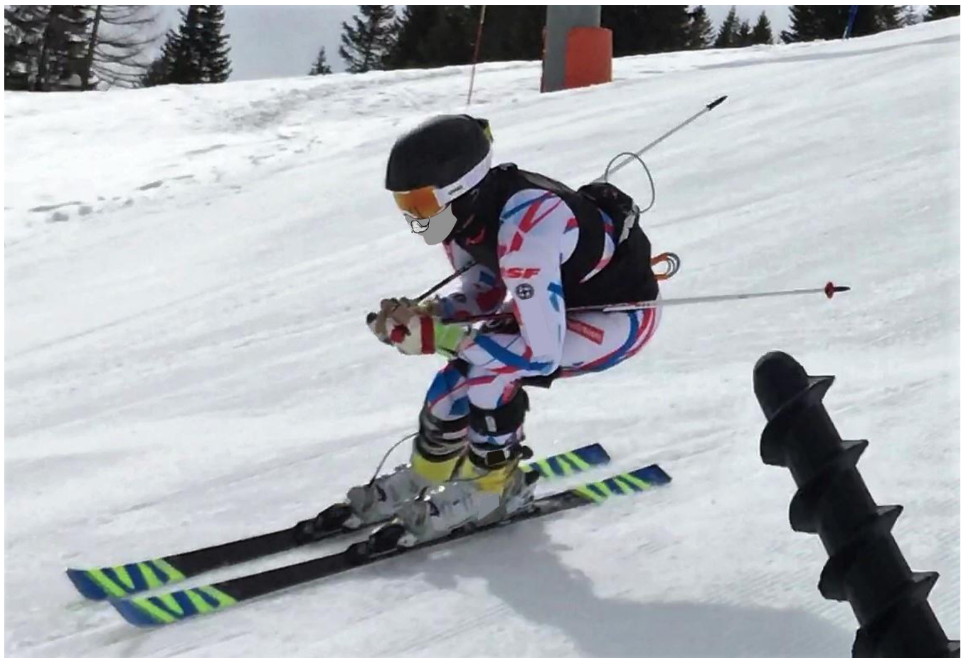
Fig 1. Skier equipped with experimental technology. Pictured is a skier performing a trial, while equipped with boot-mounted force platforms, wired to an acquisition card carried in a small bag around the waist with a GNSS unit secured inside.
