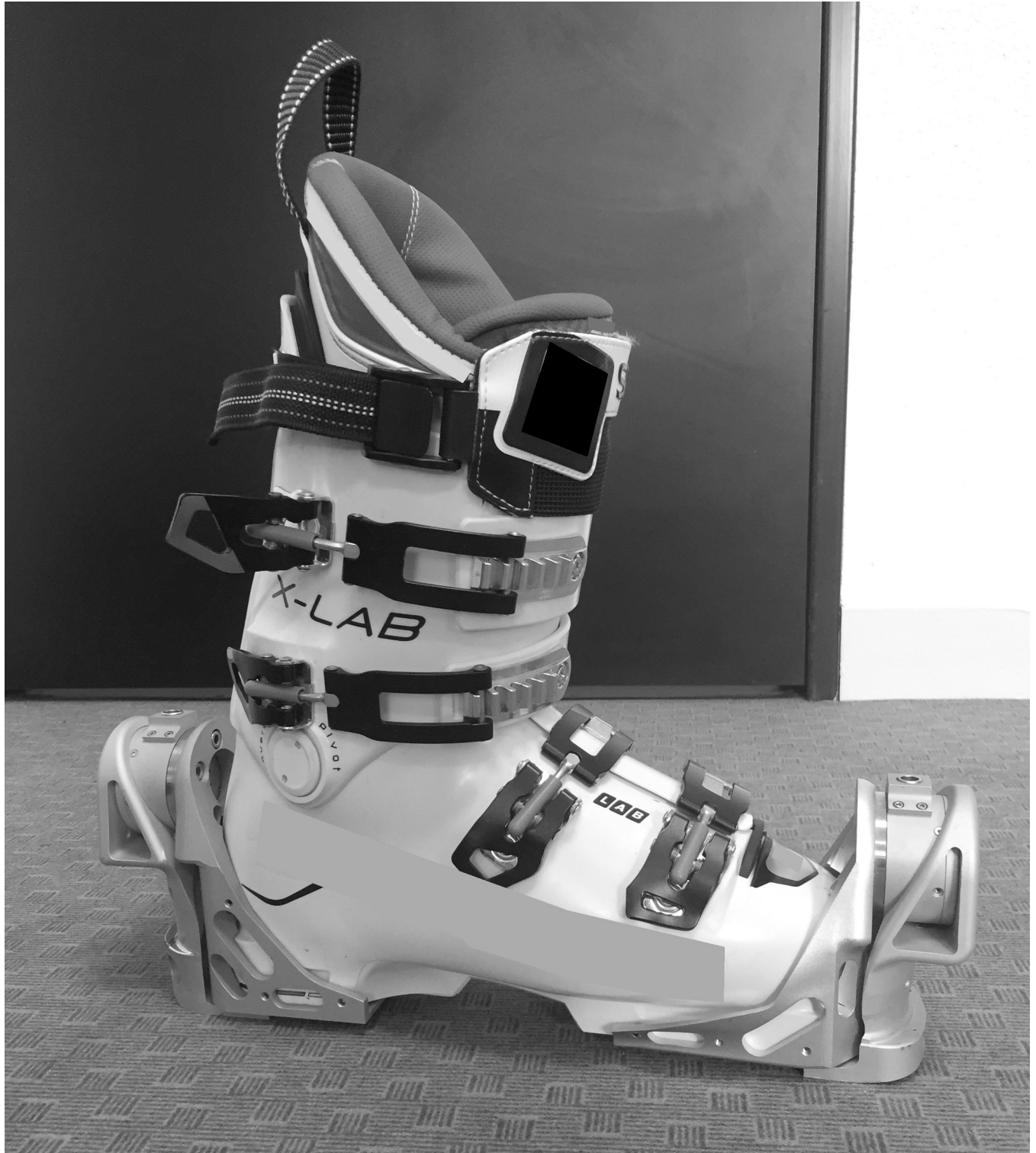
Fig 3. Ski-specialized force plates. Pictured are the specialized force-plate devices used to collect the primary SRF data in this study, attached to a pair of standardized boots used during the experiment. The novelty of these devices in contrast to previous designs is that the circular strain gauges are situated at the front and rear of the boots, where they are affixed between two 'floating' metal brackets as the only point of connection between the skier and the ski. This shift in the placement of the strain gauges enabled clip-in height to be minimized, and the mass to be reoriented more distally compared to previous iterations. Each force plate could provide force and moments in three axes (medio-lateral = x, antero-posterior = y, normal = z), but only resultant forces were examined in this study.
