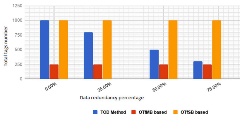
Fig 12. TOD method vs the OTfMB and OTfSB approaches: The number of tags generated against data redundancy percentage, K = 1000 , total number of blocks in a data file, 4 Data Blocks are used in generating one tag in OTfMB approach.
