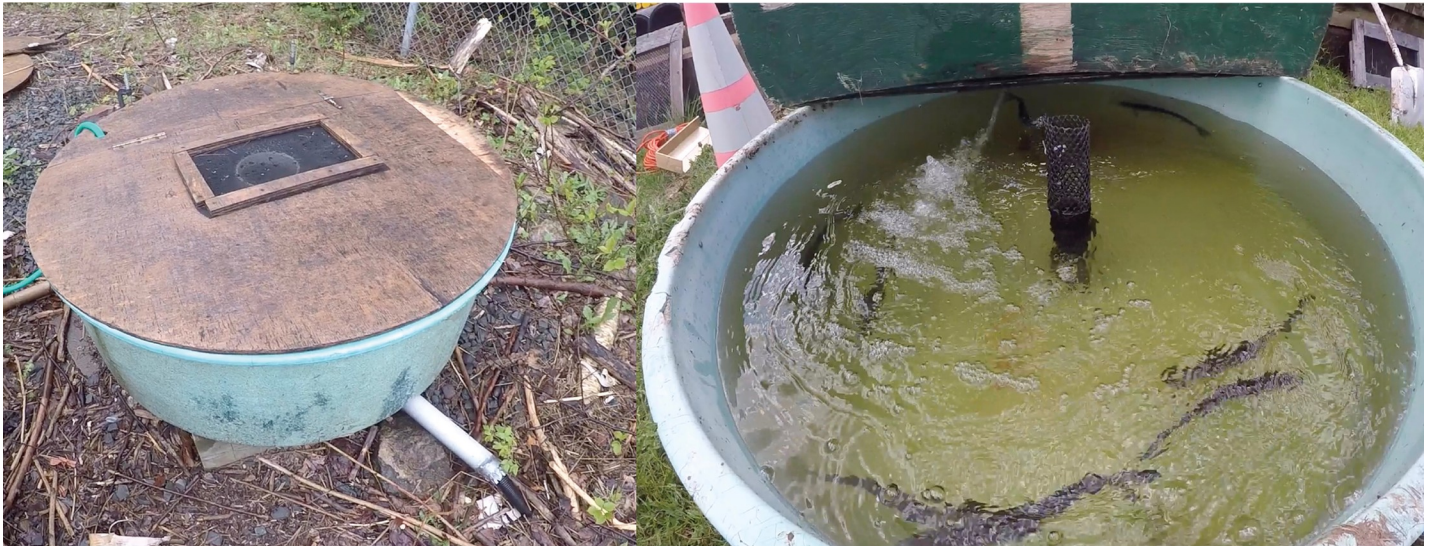
Fig 2. Pictures of holding tank (270 L) used to retain alewives during field trials at the White Rock Fish Ladder, Gasperau River, Nova Scotia. Both the holding and recovery tanks were analogous and located outdoors near the fish ladder on Nova Scotia Power Inc property.
