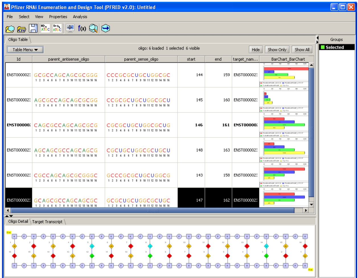
Fig 3. PFRED user interface. The main “Oligo Table” stores all the data generated through the oligo enumeration workflow (oligo sequences with their properties) and provides access to common spreadsheet functions. It is possible to assign selected oligo sequences to specific groups which can be shown and accessed under “Groups” on the right-side panel. More detailed information about the oligo sequence notation and the primary mRNA transcript can be visualized at the bottom of the user interface by enabling the “Oligo Detail” and “Target Transcript” panels.
