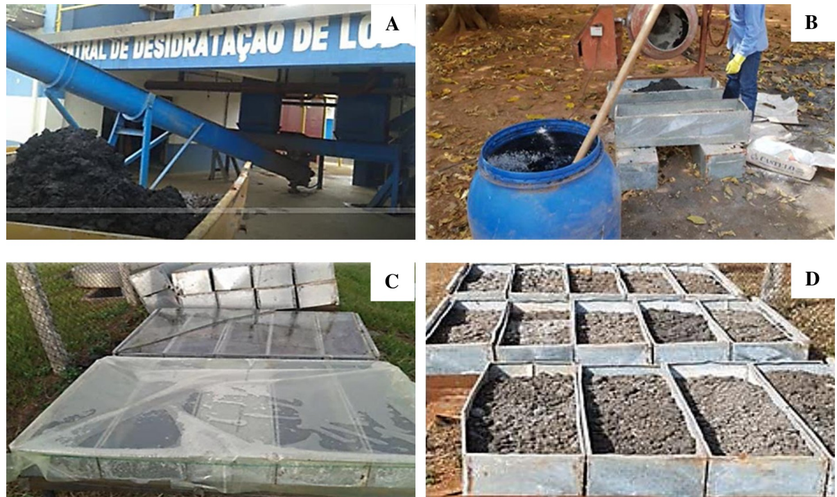
Fig 1. Process of sewage sludge treatment. A. solid residue after centrifugation; B. treatment with hydrated lime; C. exposure to sunlight; D. drying in the sun.
