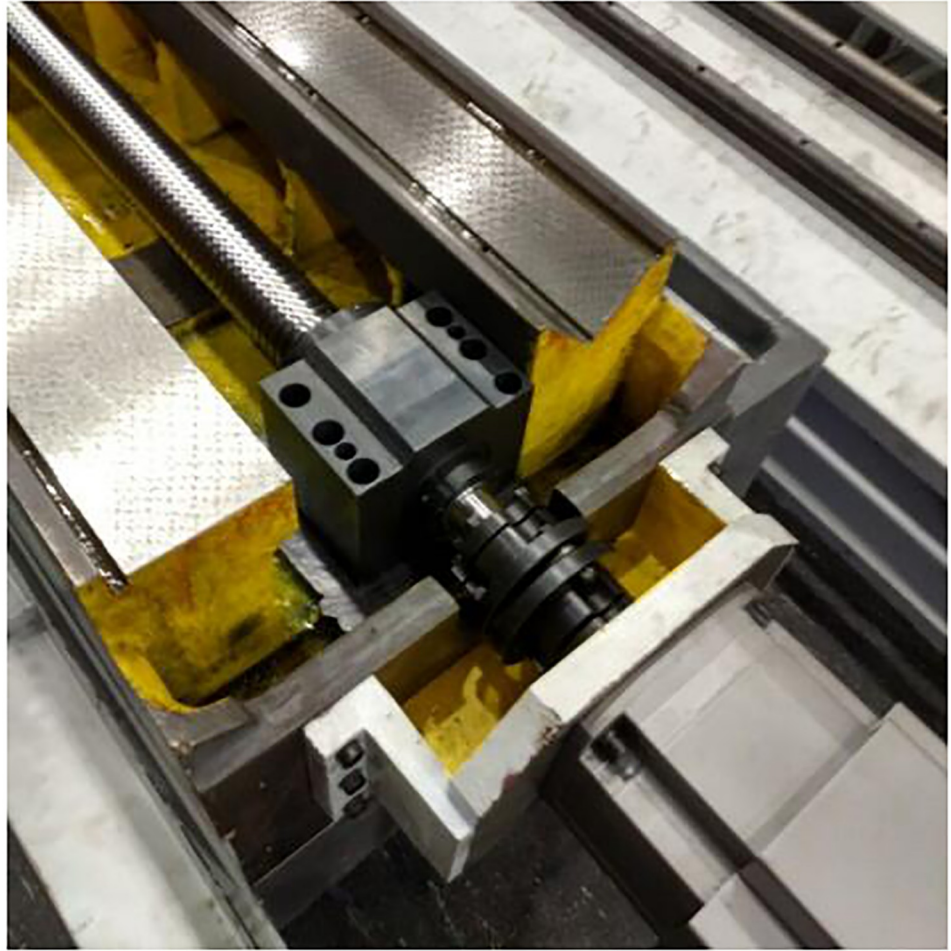
Fig 11. Reconditioned grinding machine feed system.
