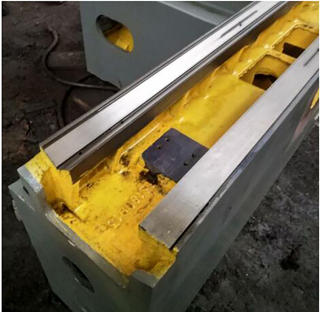
Fig 8. Reconditioned grinding machine integrated guideway.
