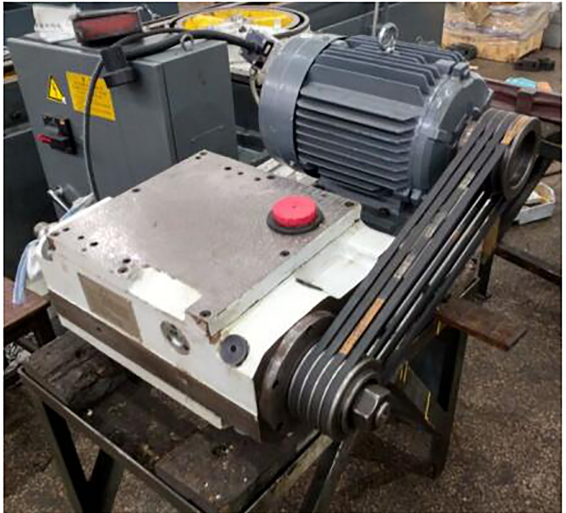
Fig 9. Reconditioned grinding wheel frame spindle system.
