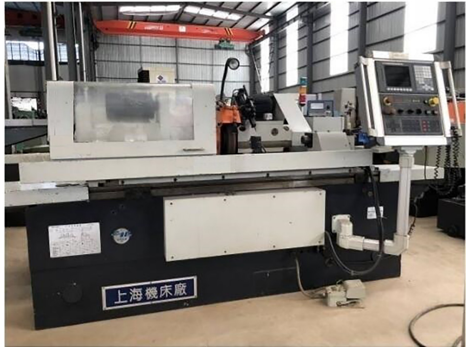
Fig 14. The remanufactured M1332B cylindrical grinding machine.
