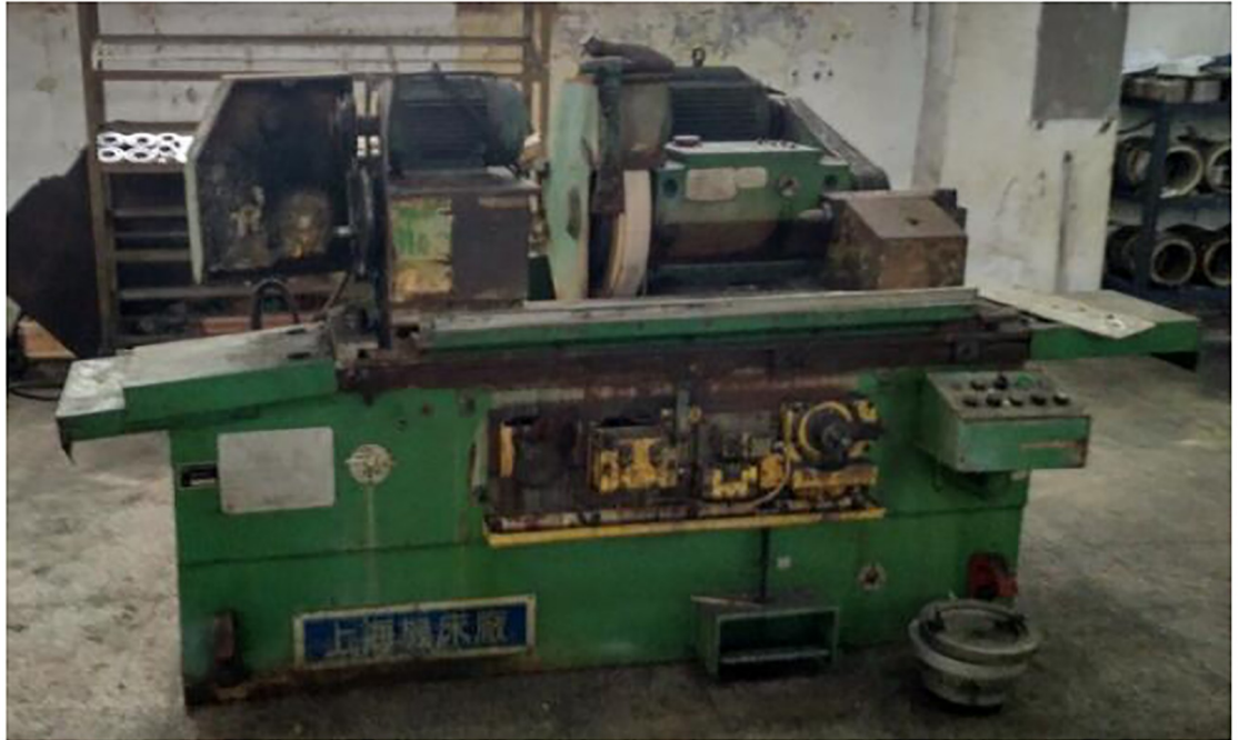
Fig 7. The retired M1332B cylindrical grinding machine.
