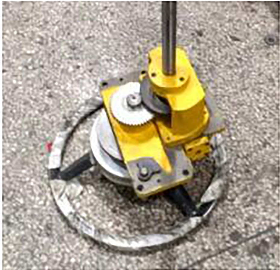
Fig 10. Grinding machine feed system before reconditioning.
