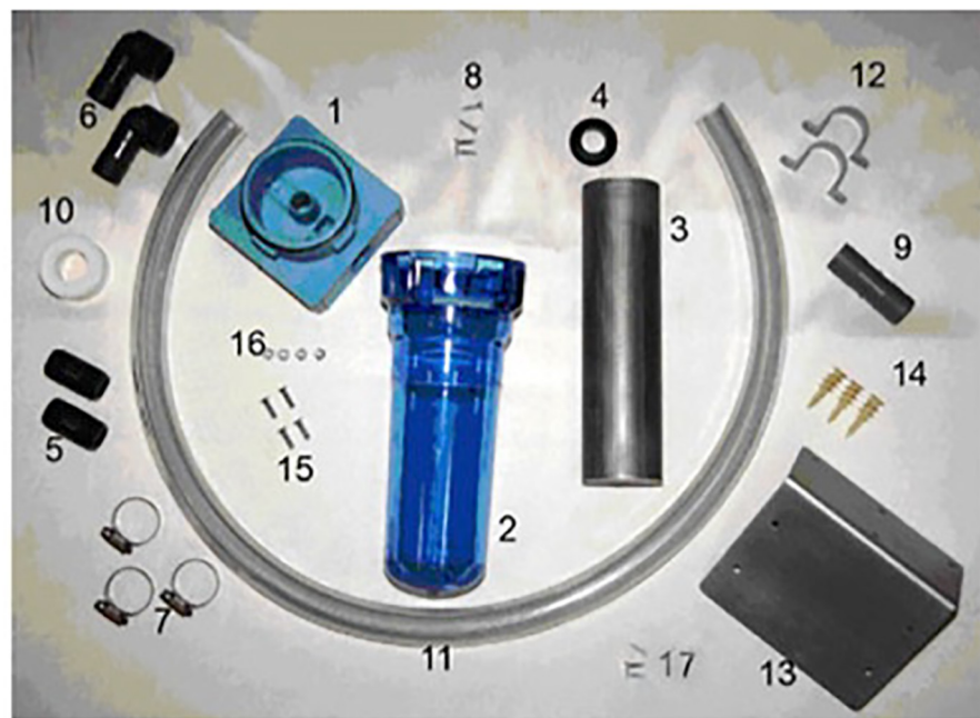
Fig 1. Composition of the washing-machine filter. This includes a filter-head (1), filter case (2), stainless steel filter of either 2 mm or 150 µm pores (3), rubber grommet (4), 19 x 51 mm pipe nipples (5), 19 mm female x 25 mm barbed hose with a 90° elbows (6), stainless steel clamps (7), wood-screws (8), 25 mm barbed tube (9), polytetrafluoroethylene tape (10), 25 x 1000 mm hose (11), 25 mm conduit clamps (12), metallic angled mounting bracket (13), drywall anchors (14), 19 mm machined screws (15), machined screw nut (16), 19 mm wood screws 19 mm. This picture was provided with permission from B. Jollimore at www.environmentalenhancements.com .
