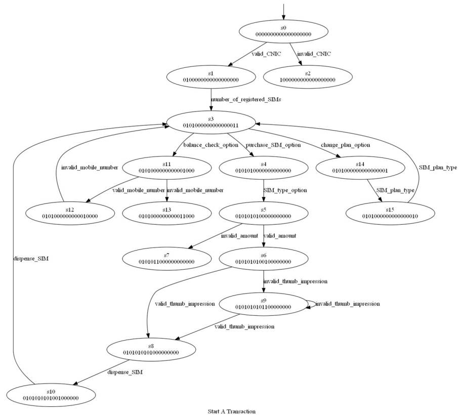
Fig 11. A SIM vending machine start a transaction Kripke structure.
