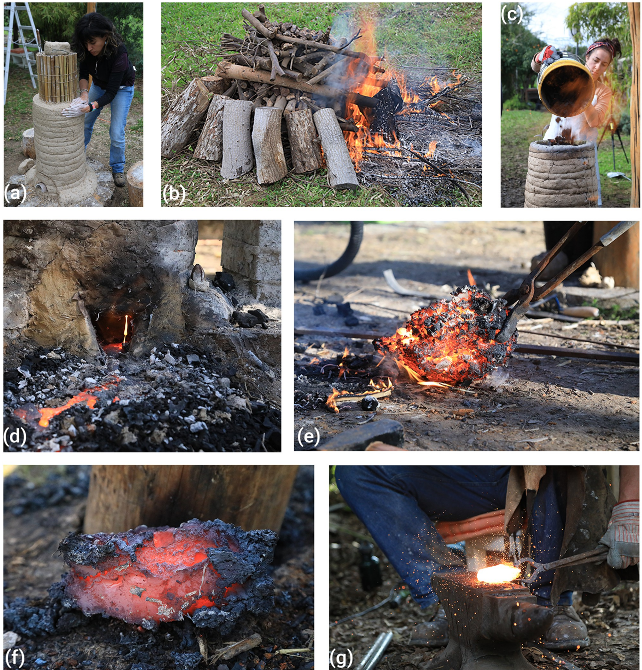
Fig 3. Various stages of field smelting experiments. (a) Building the shaft furnace using clay and bamboo, (b) Ore roasting, (c) Loading the furnace with charcoal during smelting, (d) Tapping the slag, (e) Removing the bloom from the furnace when red hot, (f) View of the bloom after being sectioned into four part while still red hot (g) Smithing the bar on an iron anvil.
