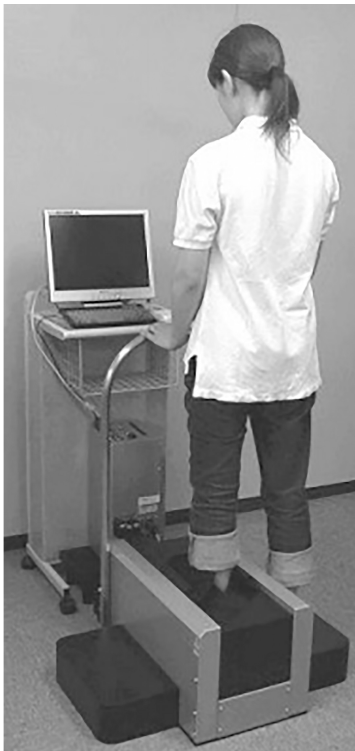
Fig 3. Infot ® scanner. Scanner used to obtain the foot scans.
