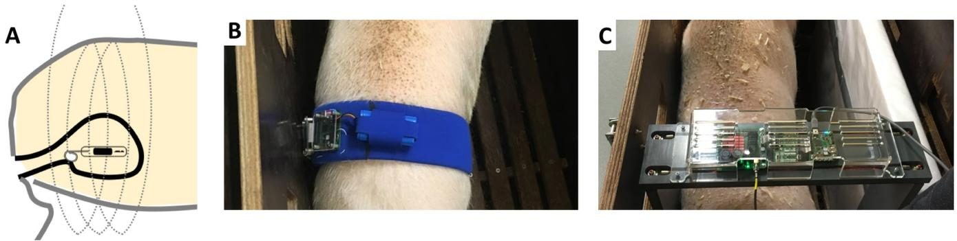
**Fig 2. Principle of Bladder Pill for pressure measurement in animals.** (A) Diagram of working mechanism of Bladder Pill in vivo, wireless induction as represented by coils (dotted lines) contained within a corresponding external device. (B) Waistband-form external device tested in vivo. (C) Rectangular frame.
