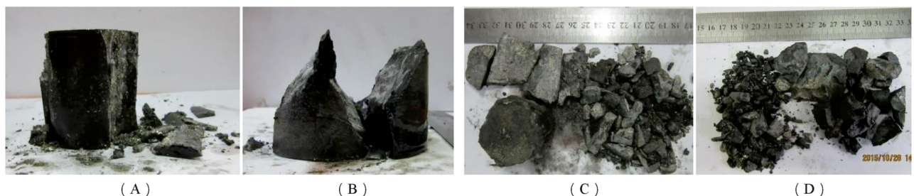
Fig 22. Failure mode of deep serpentine under different preload axial pressures (confining pressure of 20 MPa). (A) Axial compression 100 MPa; (B) Axial compression 120 MPa; (C) Axial compression 140 MPa; (D) Axial compression 160 MPa.
