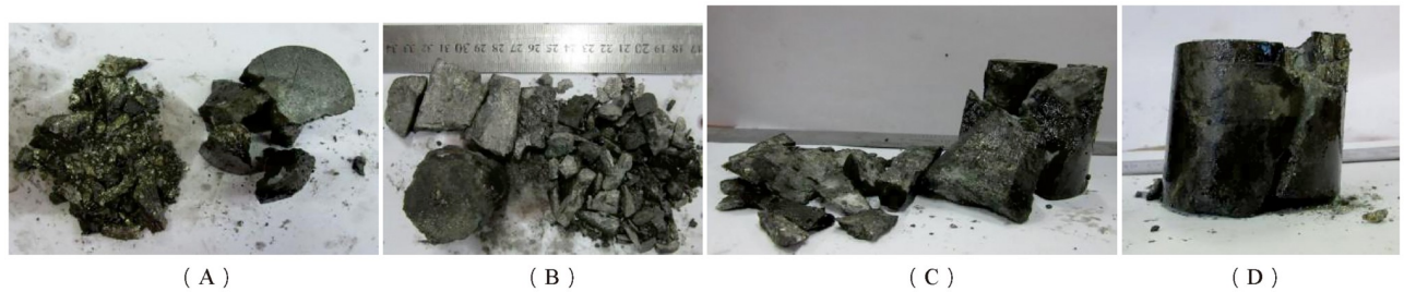
Fig 23. Failure mode of deep serpentinite under different preloaded confining pressures (axial compression of 140 MPa). (A) Confining pressure 15 MPa; (B) Confining pressure 20 MPa; (C) Confining pressure 25 MPa; (D) Confining pressure 30 MPa.
