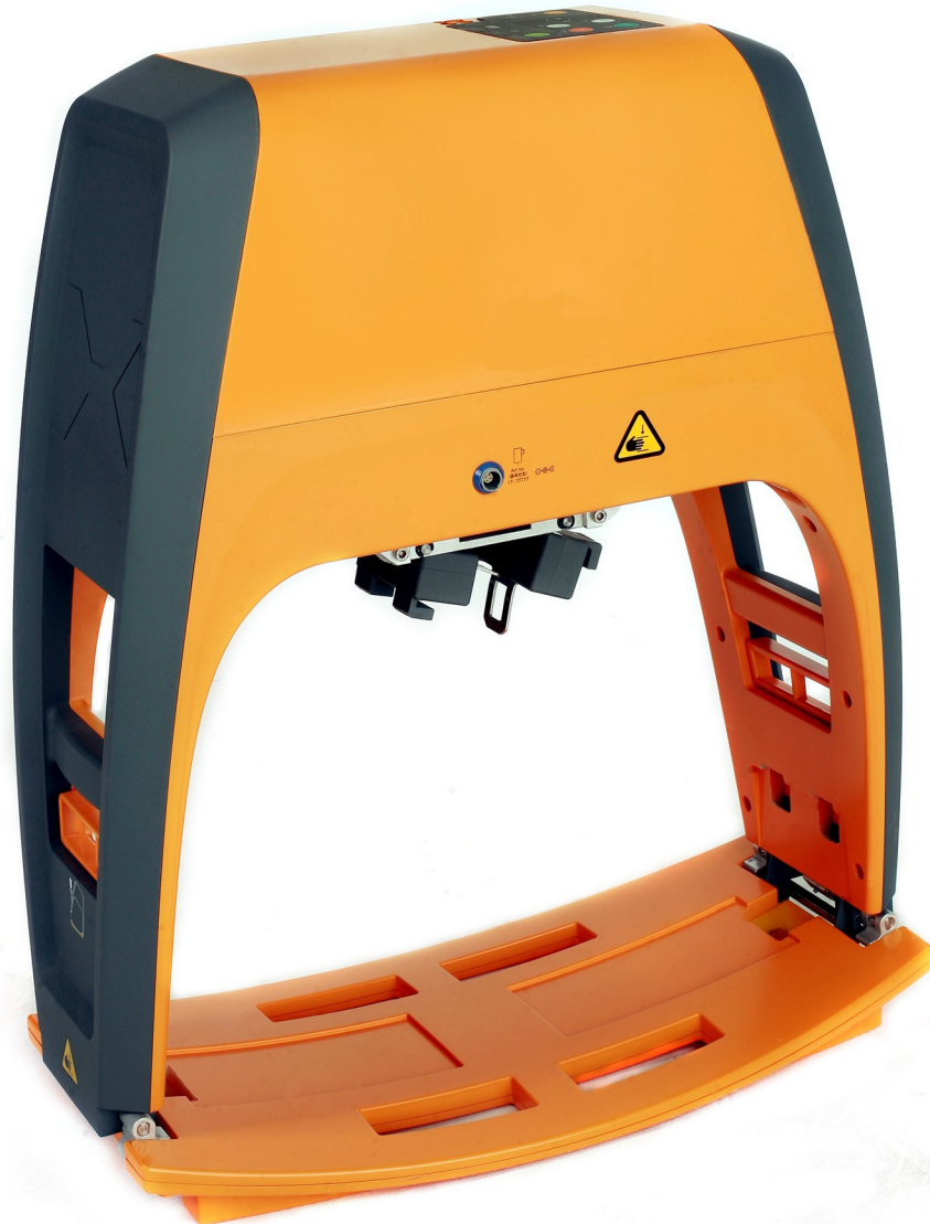
Fig 1. Automatic SST-CPR device (X-CPR). The main compression unit is positioned at the top of the device, which is operated by a battery-powered motor. The strap is attached to both sides of the central piston.
