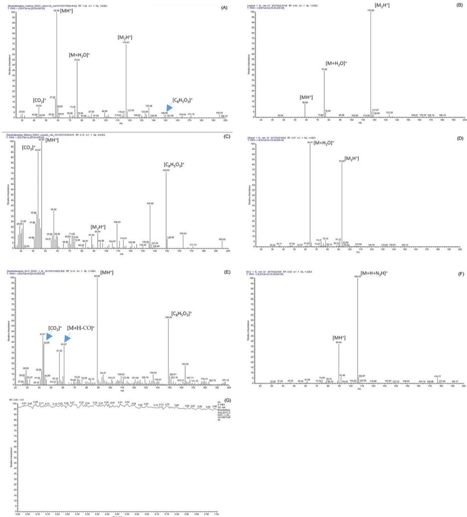
**Fig 12. Mass spectra of the needle-to-post and the UV lamp ion sources.** (A) Acetone, needle-to-post ion source; (B) Acetone, UV lamp ion source; (C) Ethanol, needle-to-post ion source; (D) Ethanol, UV lamp ion source; (E) Ethyl acetate, needle-to-post ion source; (F) Ethyl acetate, UV lamp ion source; (G) Ethyl acetate, needle-to-post ion source.
