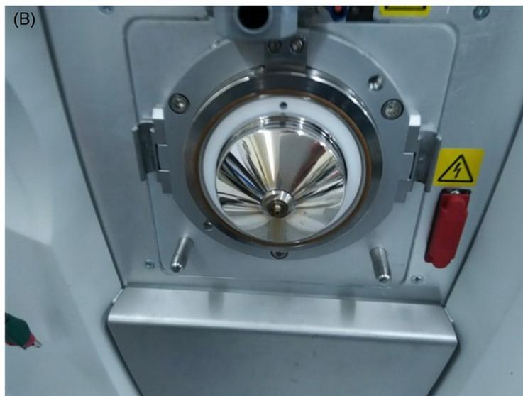
**Fig 4. Block diagram of needle-to-post ion source for mass spectrometry.** (A) Schematic of experiment system; (B) Thermo Scientific LTQ XL ion trap mass spectrometer.
