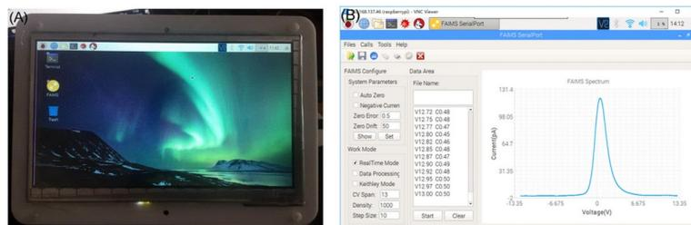
**Fig 15. The detection system based on QT.** (A) The hardware; (B) The FAIMS spectra.
