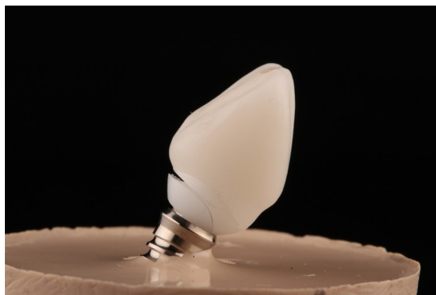
Fig 6. Fracture in the abutment of the Z-LD group.
