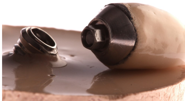
Fig 5. Fracture in the fixing screw of the T-CM group.
