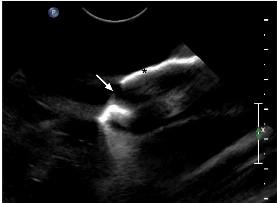
Fig 4. Ultrasound image of model C immersed in water. Model C made of nylon PA 12 using an EOS Formiga P100 printer and selective laser sintering printing technology. Note the characteristic hyperechoic appearance created by the strong reflection of the ultrasound beam by the model, simulating bone (*). The joint space is visible as a gap between the cranial (left) and caudal (right) articular processes (white arrow).
