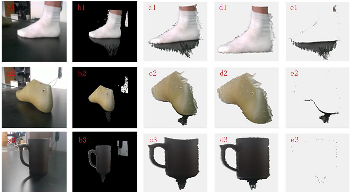
Fig 7. Point cloud filtering results with different reflective surfaces: (a1~a3): RGB images of Reflective surface 1, Reflective surface 2 and Reflective surface 3; (b1~b3): RGB mapping images of Reflective surface 1, Reflective surface 2 and Reflective surface 3; (c1~c3): Original point cloud with color of Reflective surface 1, Reflective surface 2 and Reflective surface 3; (d1~d3): Point cloud with color after filtering of Reflective surface 1, Reflective surface 2 and Reflective surface 3; (e1~e3): Removed point cloud with color of Reflective surface 1, Reflective surface 2 and Reflective surface 3.
