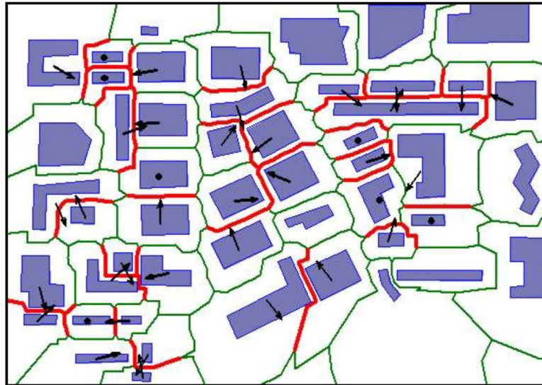
Fig 11. An illustration of the conflict skeletons, conflict OPs (Object Polygon) visualized as red lines, and the arrows represent the building movement direction.
