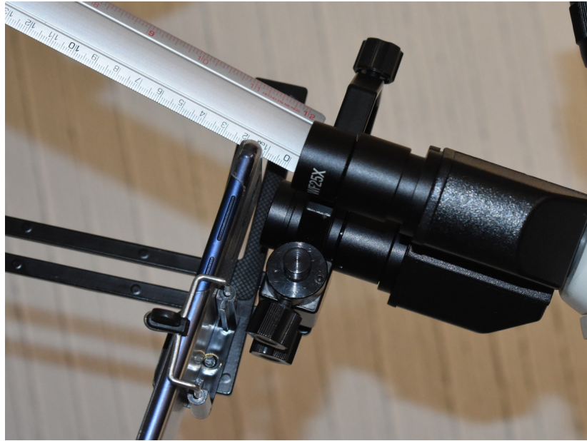
Fig 5. Distance between the microscope's ocular and the smartphone lens.
