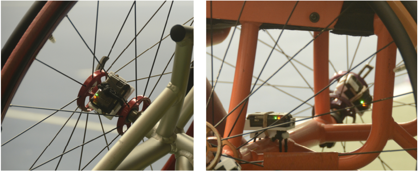
Fig 1. Placement IMUs, Left: Wheel, Right: Frame.
