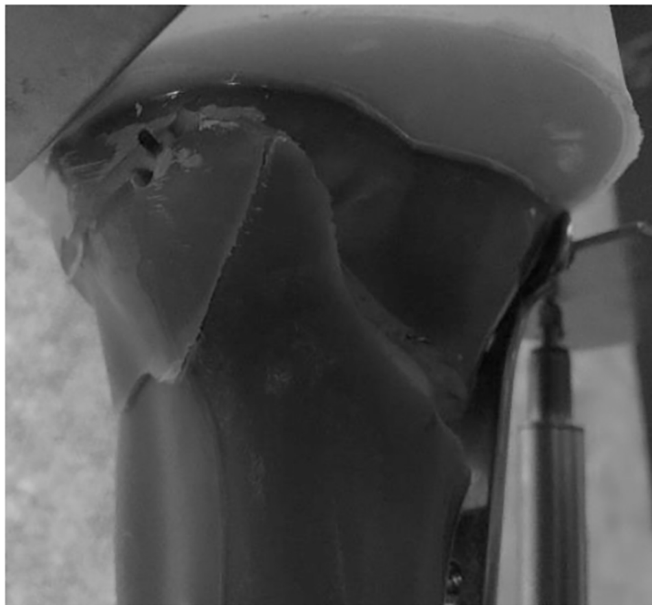
Fig 6. Example of lateral cortex fracture indicating failure of the construct.
