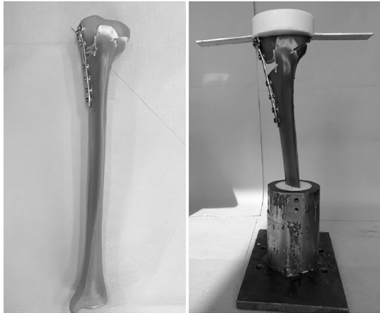
Fig 2. A specimen that has undergone MOWHTO (left) is then prepared for testing (right).
