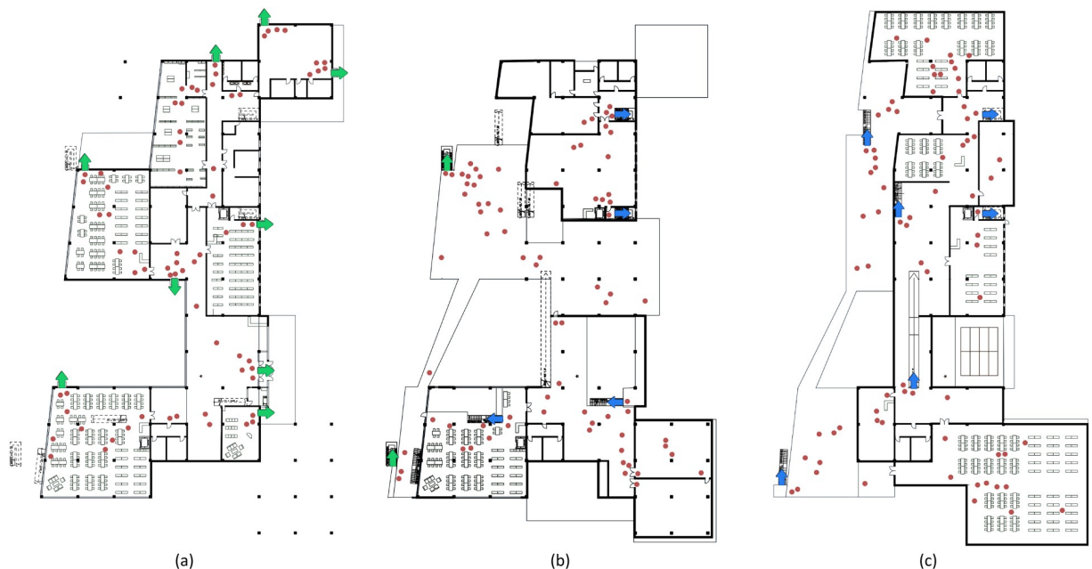
Fig 6. Evacuation process at the (a) first, (b) second, and (c) third floors.
