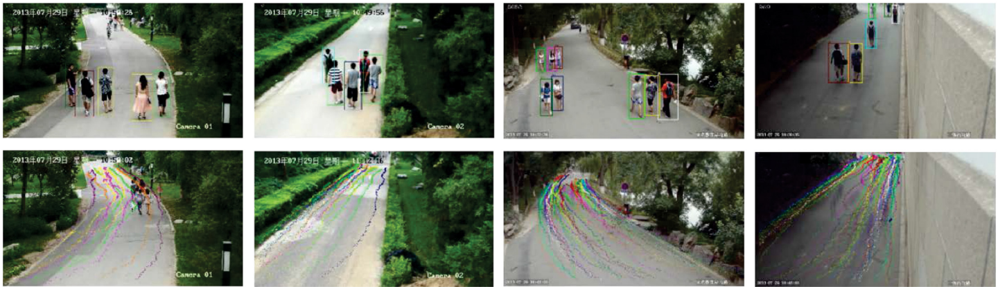
Fig 8. Examples from the PKU dataset: The first row shows sample images with labelled pedestrians in cameras HD01, HD02-1, WMHD-1 and YTX-1, and the second row shows the corresponding pedestrian centroid trajectory.
