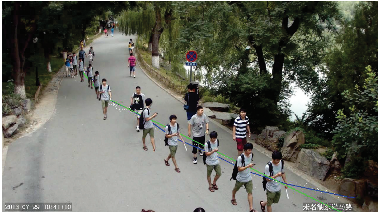
Fig 5. Illustration of the WTF algorithm by using the man wearing a grey T-shirt: The blue line represents his walking trajectory in several gait cycles, while the green one denotes the fitted walking line in the gait period. For better visualization, all his silhouette images in a gait period are manually superposed in one picture.
