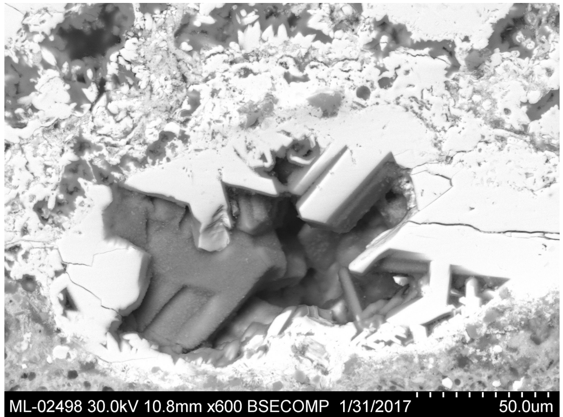
Fig 22. Secondary crystalline lead oxide within a microscopic cavity in the Blejești 1–1 sample. SEM image, backscattered electrons (S. Rovira).
