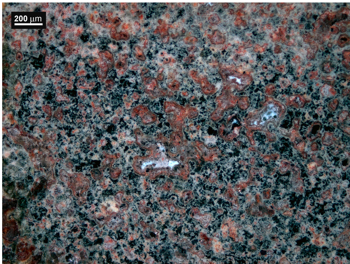
Fig 23. Appearance of the lump Blejești 1–2 core showing the colour diversity of its phases. The anglesite appears black, reddish, white and transparent crystalline. Palmierite is dispersed in clear crystalline form. OM image, Dark Field (S. Rovira).
