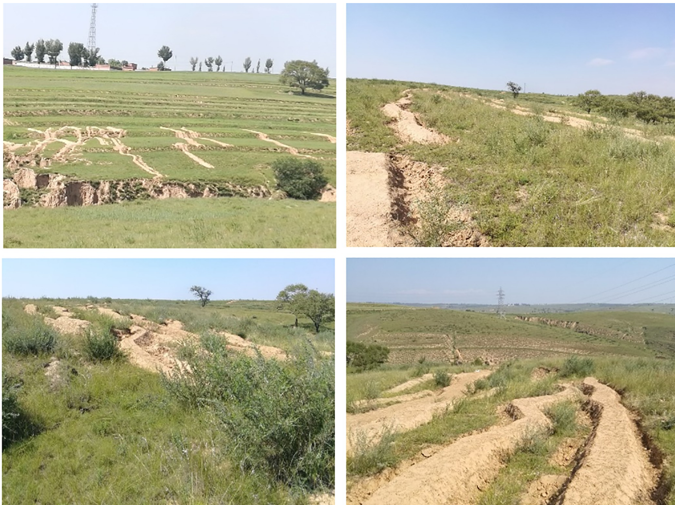
Fig 8. Ground fissures after loess filling.
