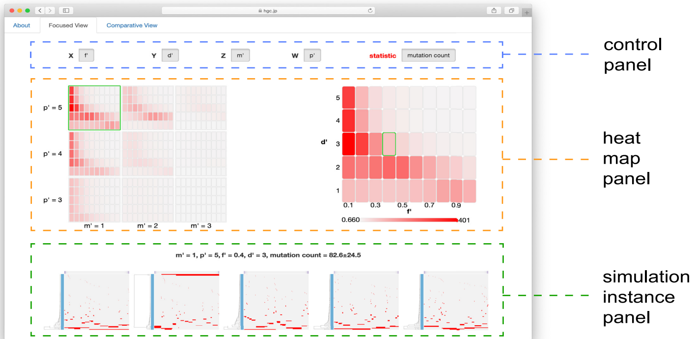
Fig 4. Focused view mode of the MASSIVE viewer. The page of the focused view mode consists of control, heat map and simulation instance panels. The control panel specifies visualization settings, the heat map panels presents heat maps for a selected statistic, and the simulation instance panel presents 5 mutation profiles from the parameter set specified by the position of the mouse cursor on the heat maps.
