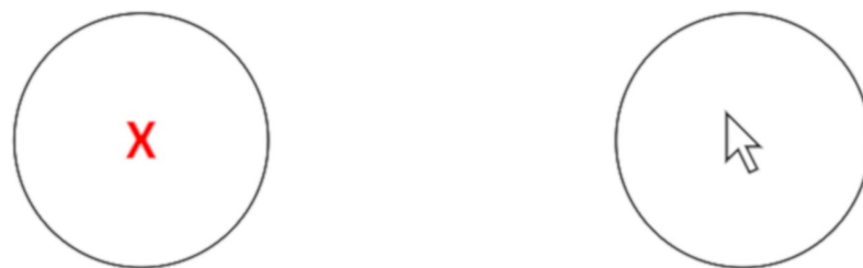
Fig 3. The Fitts' task used in this experiment. A mouse click on a blank screen began timing for each trial at which time two circles appeared. A red X appeared in 1 circle designating it the target. The participant moved to this circle and clicked within it and then as quickly as possible moved back to the previous circle (which now was the target) and clicked within it.
