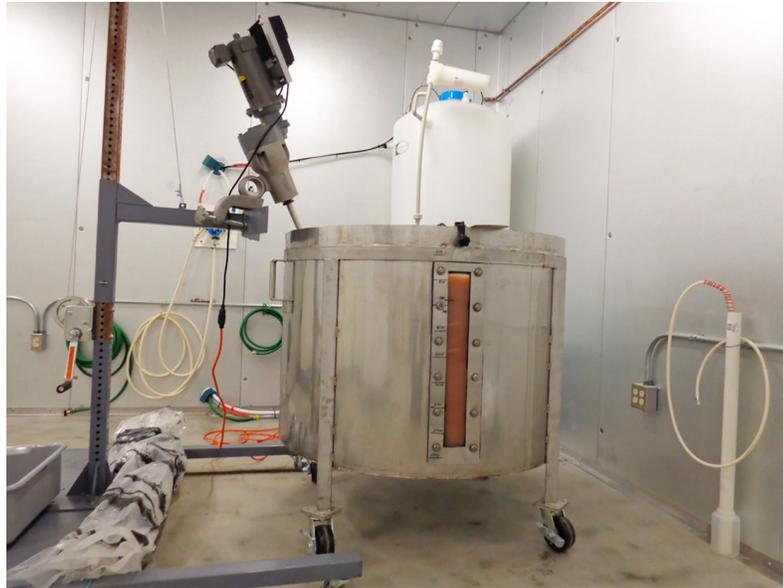
**Fig 4. 1000 L stainless steel tank containing 800 L of Cohn paste suspension.** The brown color of the suspension is visible through the window on the side of the tank. The stirring paddle can be winch-lifted out of the tank. The white tank behind the stainless steel tank holds cold ultrapure water that is recycled for 7 minutes every hour.
