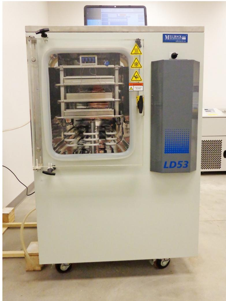
**Fig 6. Shelf-type Freeze Dryer for lyophilizing HuBChE.** Millrock Technology, model LD53S3, Kingston, NY.
