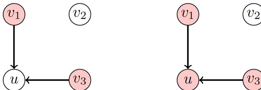
Fig 2. Illustration of the Linear Threshold model. The white colored nodes are in an inactive state whereas the pink colored nodes are in an active state. Node u will be activated if p_{v_1,u} + p_{v_3,u} \geq \theta_u .
