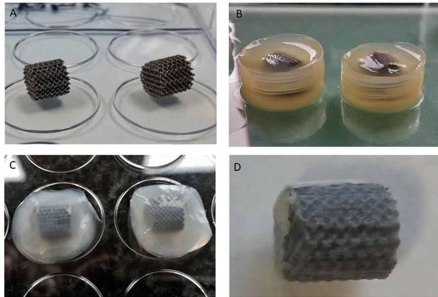
**Fig 1. Stages of preparation of BC-coated Ti6Al7Nb scaffold.** (A)—native Ti6Al7Nb scaffold; (B)—implant coated with unpurified BC; (C)—BC-coated implant after removal of media leftover and bacteria; (D)—BC-coated Ti6Al7Nb scaffold after partial drying.
