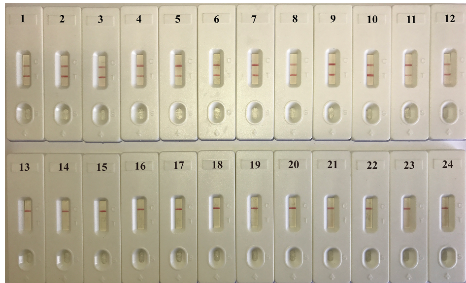
Fig 5. Specificity of the K. pneumoniae -MCDA-LFB assay. Biosensor 1, K. pneumoniae (ATCC2146). Biosensors 2–6, different K. pneumoniae strains from sputum. Biosensors 7–8, different K. pneumoniae strains from urine. Biosensors 9–12, K. pneumoniae strains from blood, pharyngeal swabs, puncture fluid, and wounds, respectively. Biosensors 13–24, Aeromonas caviae , Bacillus cereus , Citrobacter braakii , Corynebacterium stationis , Enterobacter sakazakii , Enterotoxigenic Escherichia coli , Listeria monocytogenes , Salmonella enterica , Shigella flexneri , Staphylococcus aureus , Streptococcus pneumoniae , and Streptococcus suis . MCDA, multiple cross displacement amplification; LFB, gold nanoparticle lateral flow biosensor.
